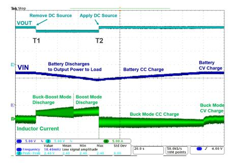
Figure 7. Battery charge/discharge operation waveform
