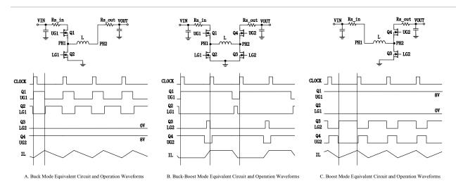
Figure 3. 4-Switch buck-boost converter operation modes and waveforms
