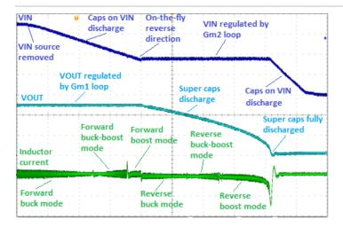
Figure 5. On-the-fly reverse-direction operation
