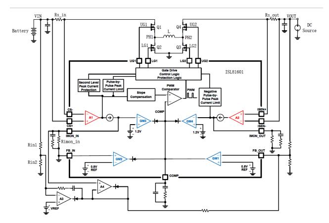
Figure 6. Battery charge/discharge CC/CV control
