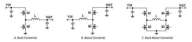
Figure 1. Bidirectional DC/DC converter topologies.
